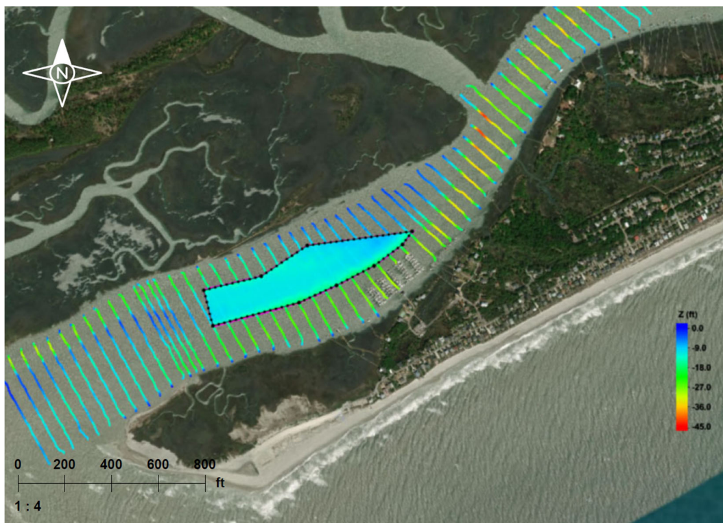
Figure 1: May 2014 bathymetric survey data with interpolated bottom surface TIN overlay.
